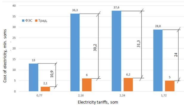
Figure 4: Comparative diagrams of electricity costs for traditional and PV grids at installed capacity of 1 MW.
