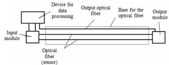
Figure 4: Structural diagram of the interference system.
