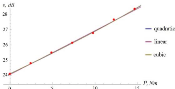
Figure 7: Loss values in the optical fiber with the wavelength of 1550 Nm with the step increment of pressure.
