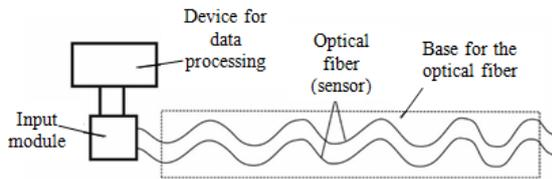
Figure 5: Structural diagram of the system based on the use of coherent optical reflectometry.
