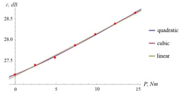
Figure 6: Loss values in the optical fiber with the wavelength of 1310 Nm with the step increment of pressure.
