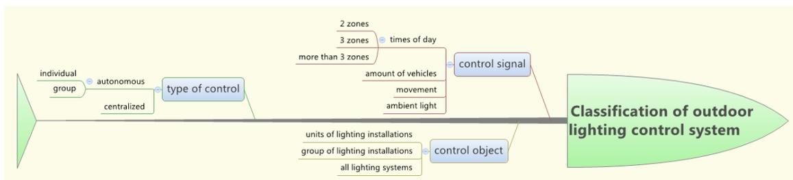
Figure 1: Classification of outdoor lighting control system.
