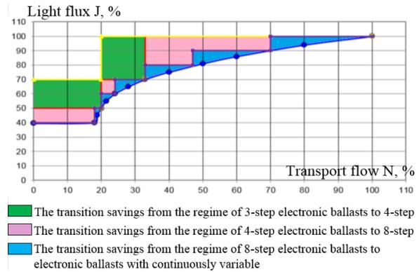
Figure 4: The application efficiency of electronic ballasts.
