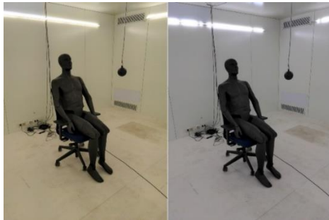
Figure 8: Experimental setup, left T1= 2600 K, right T3 = 4400 K.
