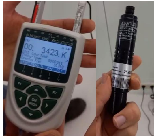
Figure 5: Color temperature sensor with device ALMEMO 2590-2.
