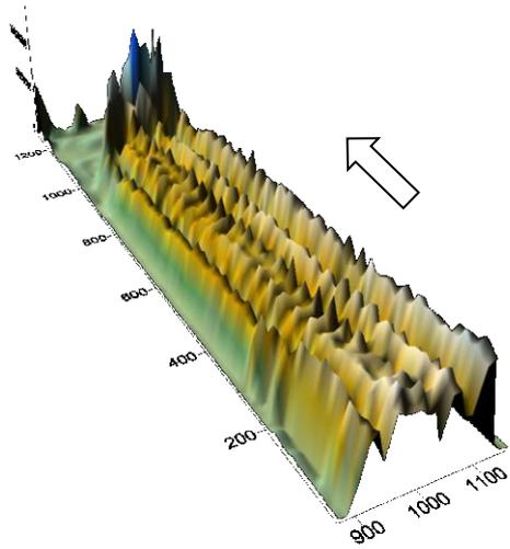
Figure 6: Ground pressure distribution along the gob: the arrow indicates the direction of the longwall advance.
