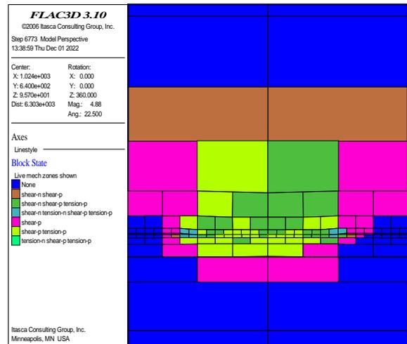
Figure 4: Damage zone distribution around the gob.
