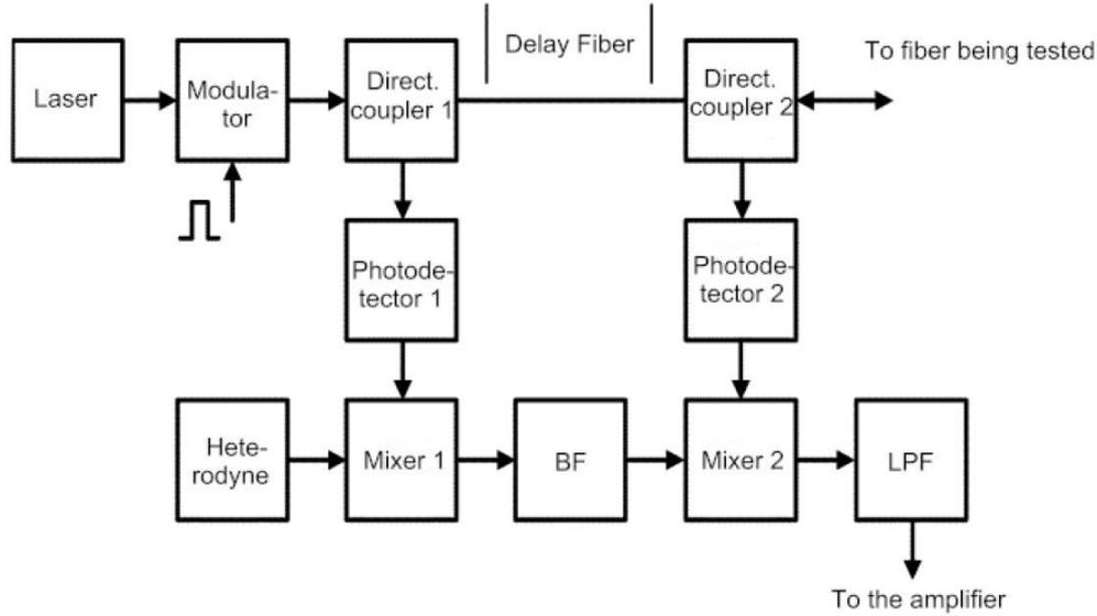
Figure 1: Schematic diagram of the frequency-difference Brillouin reflectometer.
