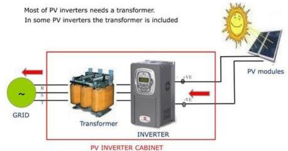
Figure 2: Appearance of the inverter.
