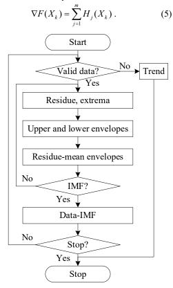
Figure 1: The block diagram of the EMD algorithm.
