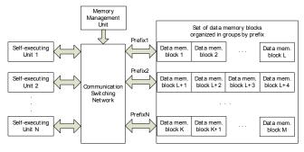
Fig. 7. Proposed model of a memory-centric system, that allows reconfigurable use of data memory blocks
