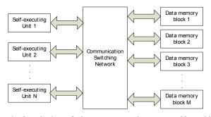
Fig. 6. Organization of the memory-centric system with multiple self-executing units
