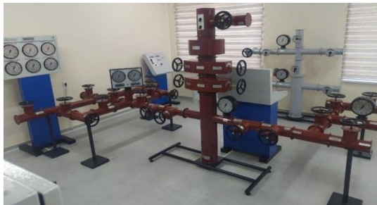
Figure 1: General view of the AMT-411 well work-over simulator.
