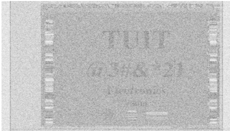
Figure 5: Intercepted and reconstructed image at the 7th harmonic (551.25 MHz).
