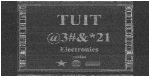
Figure 4: Intercepted and reconstructed image at the 6th harmonic (472.5 MHz).
