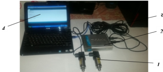
Figure 7: Process of testing the pressure recording sensor by connecting it to an analogue-to-digital converter (DAQ) and a computer.
