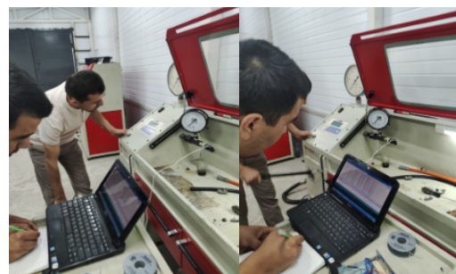
Figure 10: Process for calibrating pressure sensors with an IP40 pressure gauge.
