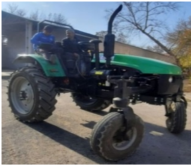
Figure 4: General view of the experimental tractor with increased maneuverability under conditions of narrow orchards and vineyards.
