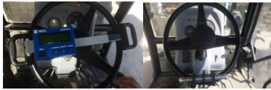
Figure 14: Measuring the force on the steering wheel rim.
