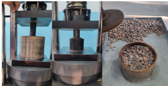
Figure 1: The process of determining the strength of expanded clay using standard cylinders.
