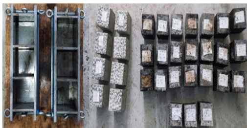
Figure 3: Prepared cube specimens and molds.
