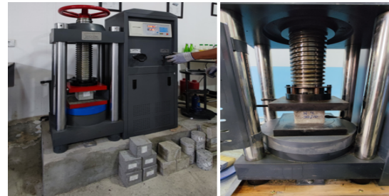
Figure 4: Compression testing process of cube specimens.
