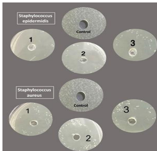
Figure 8: Antibacterial activity of AgO nanoparticles against Gram-positive bacteria at different argon flow rates.
