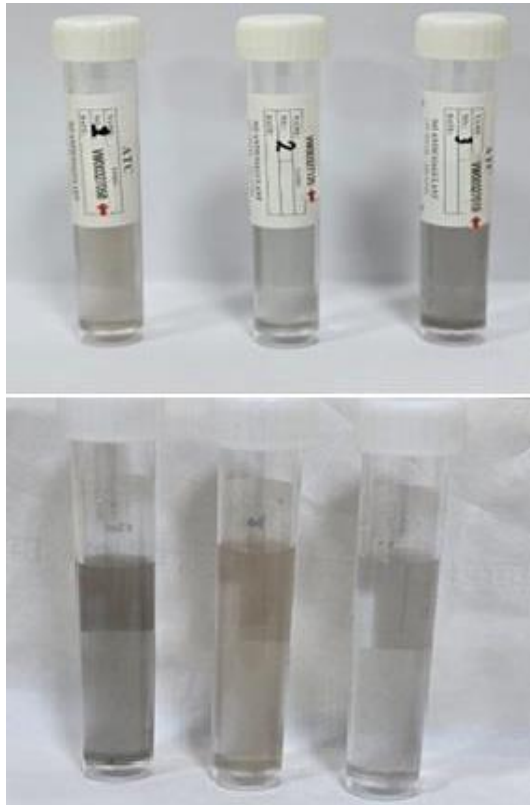
Figure 2: Plasma-assisted Ag nanoparticle suspensions prepared at different gas flow rates: (1) 0.5 L/min, (2) 1.0 L/min, and (3) 1.5 L/min.
