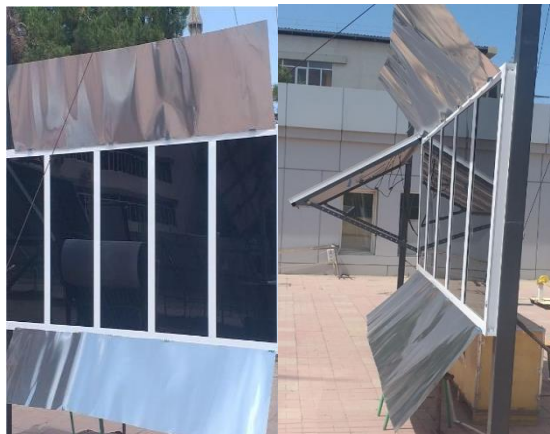
Figure 4: Photo of the vertical PV2 part of the PVI with flat reflectors made of aluminum sheet.
