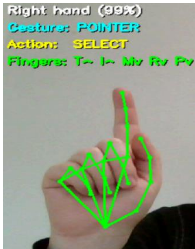
Figure 6: Pointer gesture controlling the position and hue of the LED cluster.
