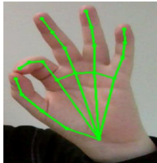
Figure 4: Example of the OK gesture turning off the LED strip.
