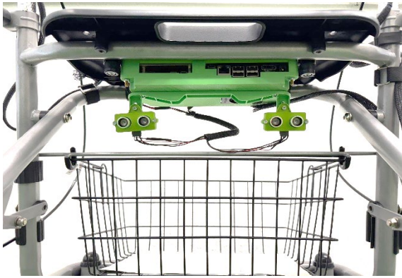
Figure 2: Housing with components fitted onto the rollator.
