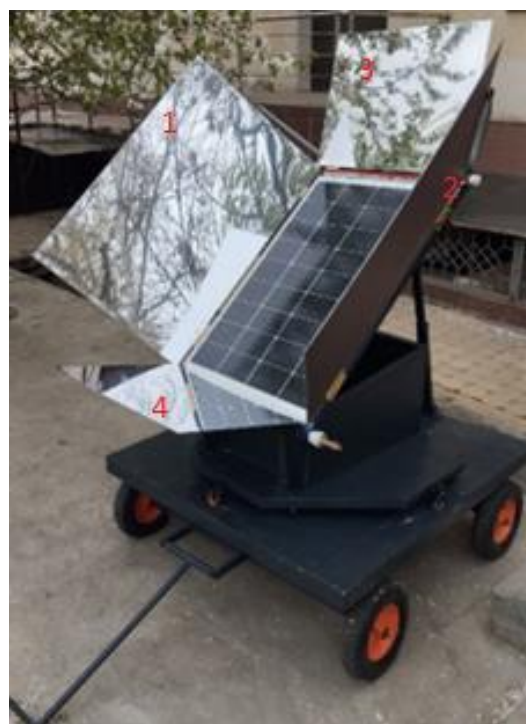
Figure 1: General view of the PVTd and reflector arrangement.
