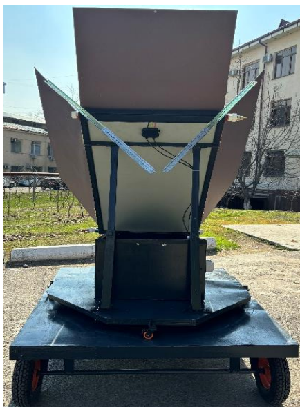
Figure 2: Structural layout of the PVT thermal collector.
