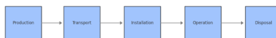
Figure 1: Stages of environmental impact assessment for Renewable Energy technologies (Life Cycle Diagram).
