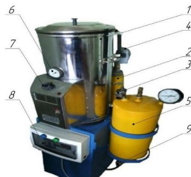
Figure 1: Small-volume biogas unit: 1 – reactor; 2 – small gasholder; 3 – burner; 4 – electric contact pressure gauge; 5 – gasholder; 6 – bimetal thermometer; 7 – temperature controller; 8 – OWEN PR 110 programmer; 9 – safety valve.
