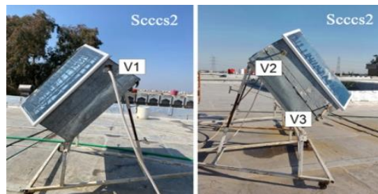
Figure 4: Shows the locations of valves V1, V2, and V3 in Scccs2.
