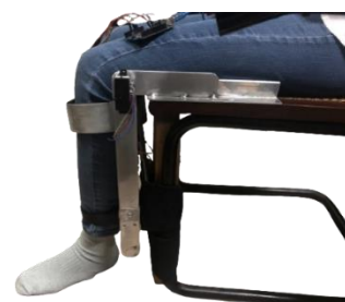
Figure 7: Experimental setup: motion intention for knee extension.
