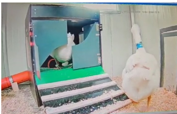
Figure 17: Goose only activates one door of the side-hinged entrance mechanism.
