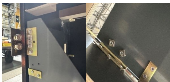
Figure 15: Magnetic stops of the side-hinged door mechanism.
