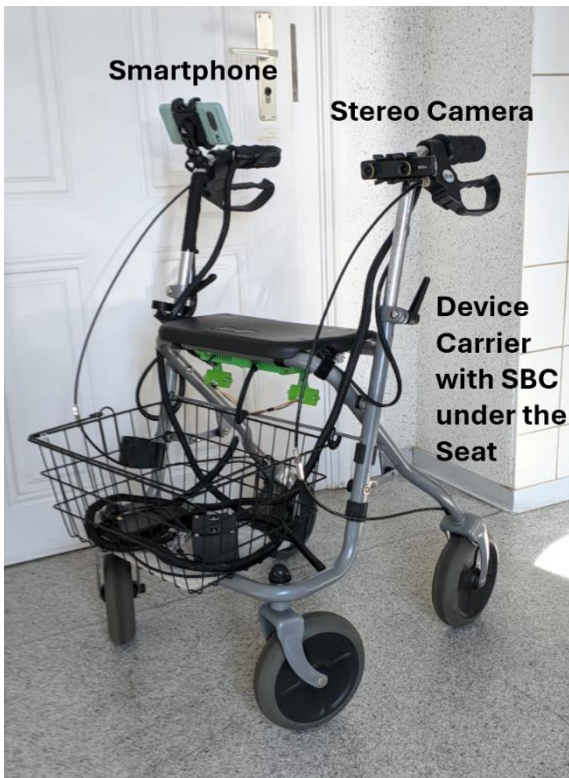
Figure 2: AktiMuW walking aid platform with stereo camera and SBC mounted under the seat.
