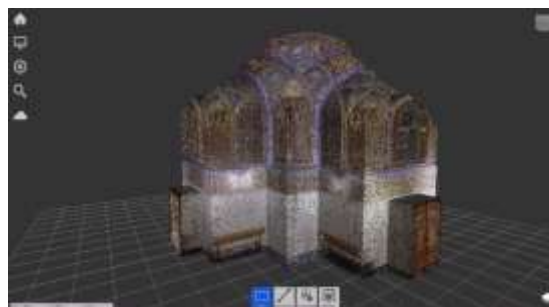
Figure 12: Three-dimensional (3D) point cloud model of the Aksaray.
