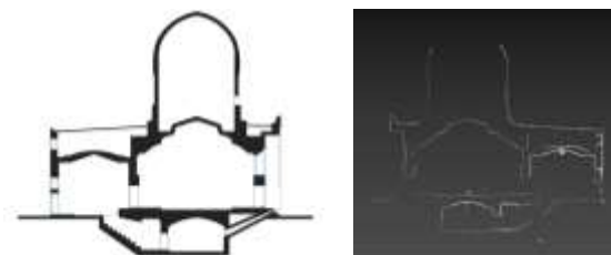
Figure 13: a) Section plan 1 drawn in Auto CAD. b) Section plan 1 from ReCap Pro.
