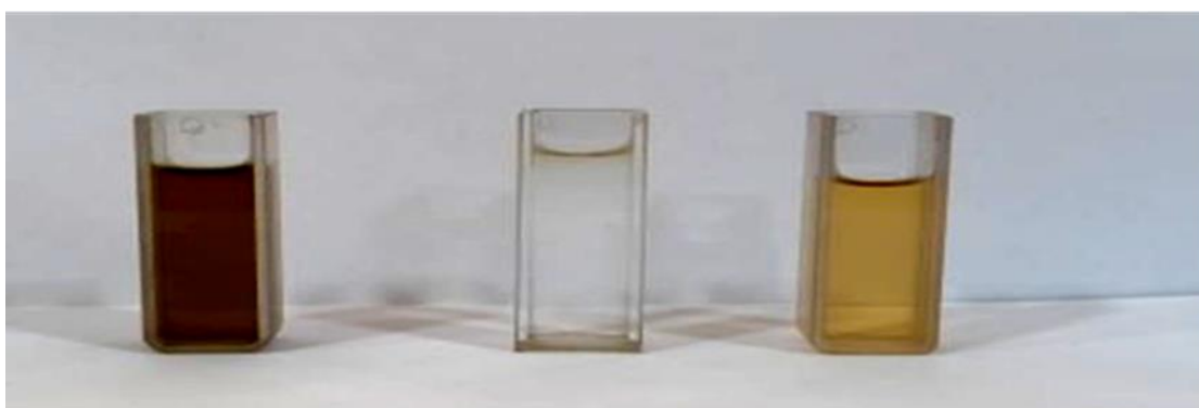
Figure 2: Synthesis of SeO NPs using \text{Na}_2\text{SeO}_3 salt as a sources of selenium metal by Camellia Sinensis dried leaves extract.
